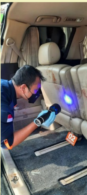
Detection of bloody fingerprint using Rofin Polilight-Flare® Plus 2 450 nm on the vehicle in Mother and Child Murder Case in Subang, West Java (August 2021).
