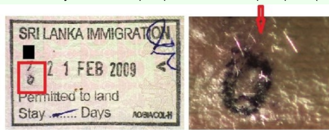
Figure 4: Fiber disturbance could be observed under side light.
