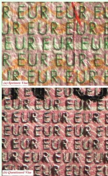
Figure 9: Micro printings observed under sidelighting (a) Raised ink of micro-printing of specimen visa (b) Embossed micro-printing of questioned visa.
