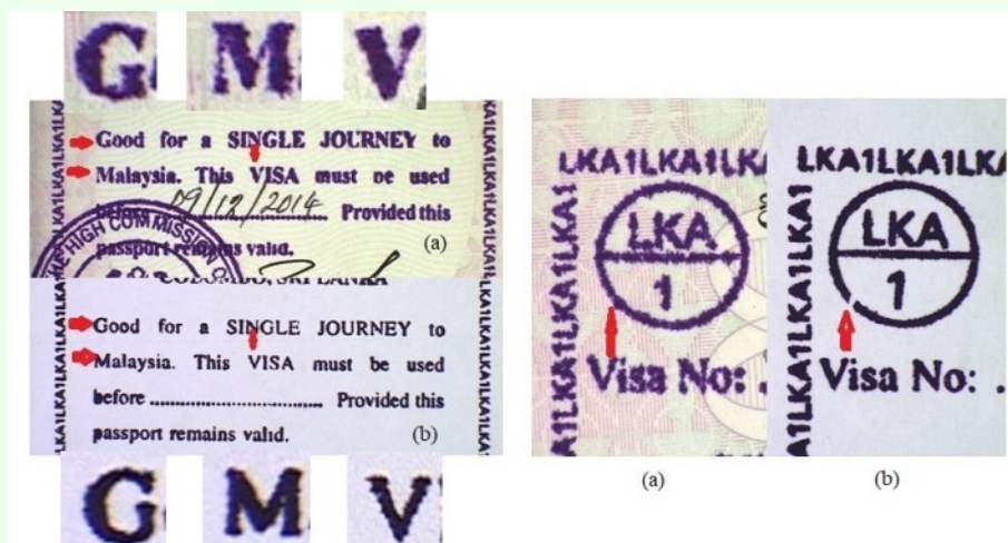
Figure 6: (a) Questioned stamp (b) Specimen stamp The arrows indicate the differences in the typefaces of both the questioned and specimen seals, as well as the gap in the specimen seal, which serves as a security feature.
