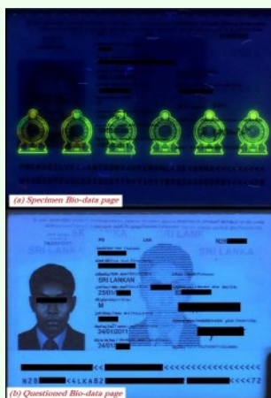
Figure 7: Fluorescence shown under UV (a) Specimen bio-data page. (b) Questioned bio-data page.
