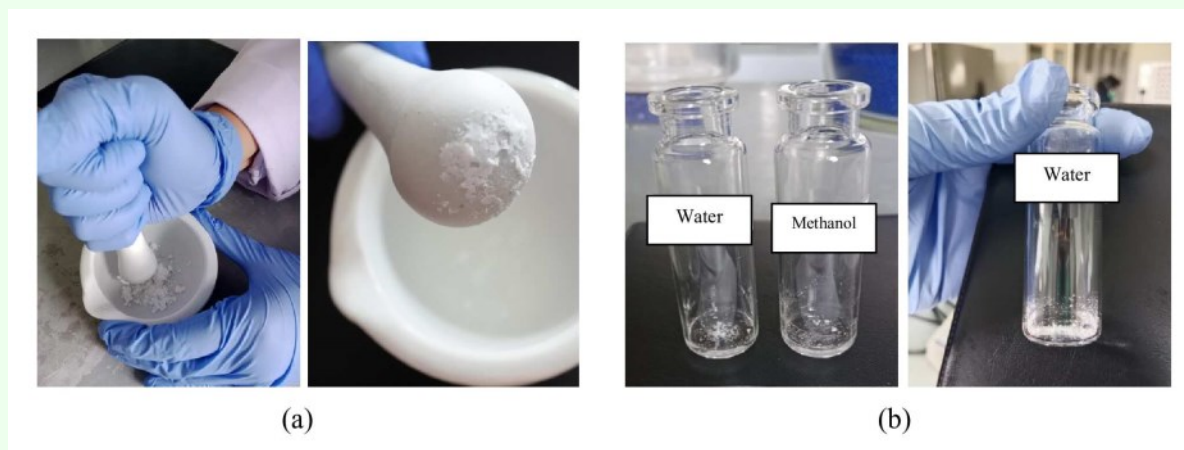
Figure 2: (a) Crushed sample; (b) Solubility test in water and methanol.
