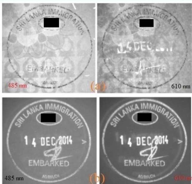
Figure 3: The questioned (a) and specimen (b) stamp impressions were observed under 485 nm and 610 nm wavelengths, (a) does not undergo any reactions (except date) as (b) does.
